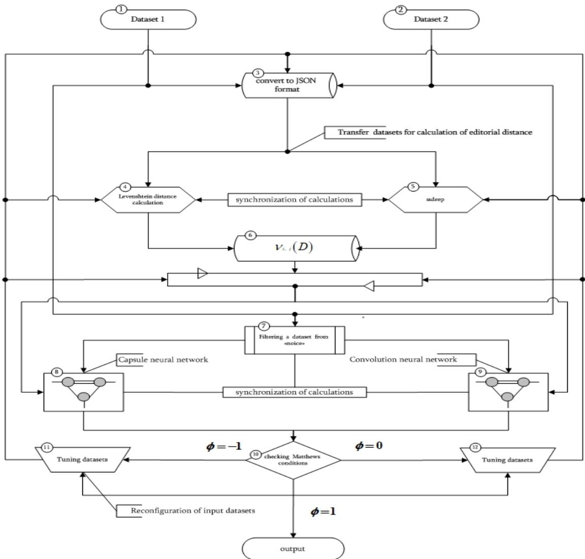
Fig. 3. Algorithm of the developed software.
